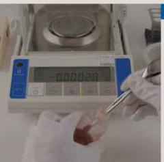
Stability and response speed should be correctly chosen according to environment and weighing objects. "Easy RES" offers the balance users very easy and simple way to change response speed. He/she can change response speed in three levels just with out-touch of SET key.
