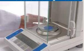
VIBRA LF series is equipped with "cross-over sliding" windshield which enables the user to open the right-side door by left-side knob, vice versa. The user can handle the weighing sample with right hand while he/she operates the door with left hand. It makes weighing operation in lab routines less time-consuming.
